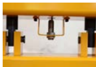
Landing detection System prevents accidental demagnetisation in the air
