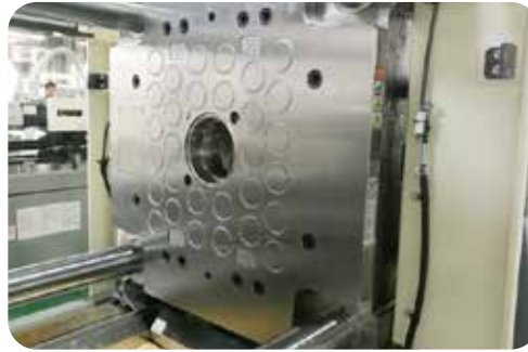
Electro permanent magnetic quick change systems for injection moulding machines and punch presses
